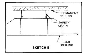
CAUTION: DO NOT ALLOW FULL WEIGHT OF UNIT TO REST ON T-BAR CEILING.
